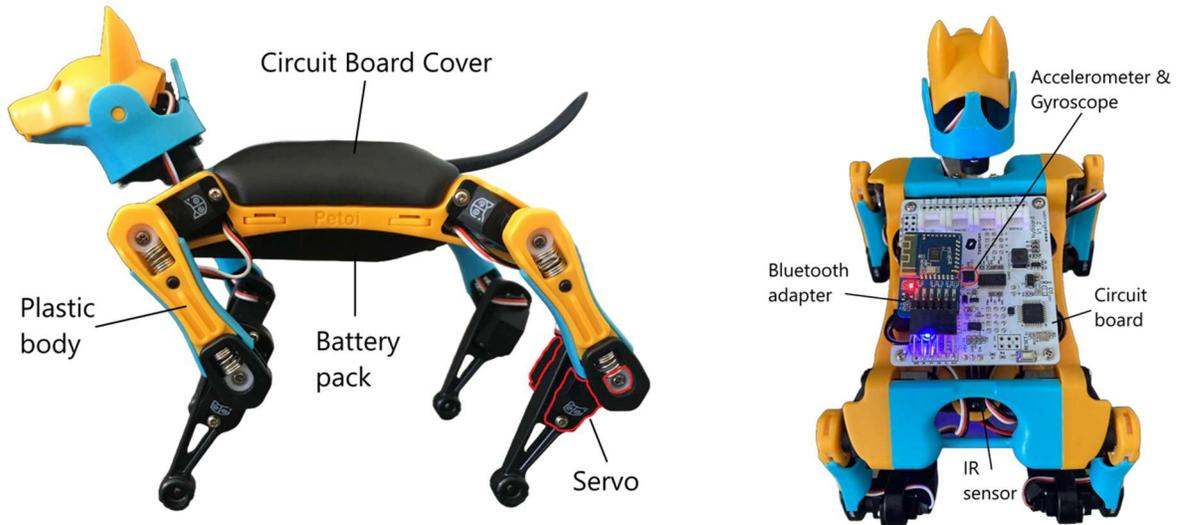
Figure 3: Labelled Diagrams of Norbert
