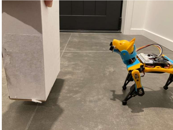
Figure 27: Using the IR Distance Sensor to Follow the Box
