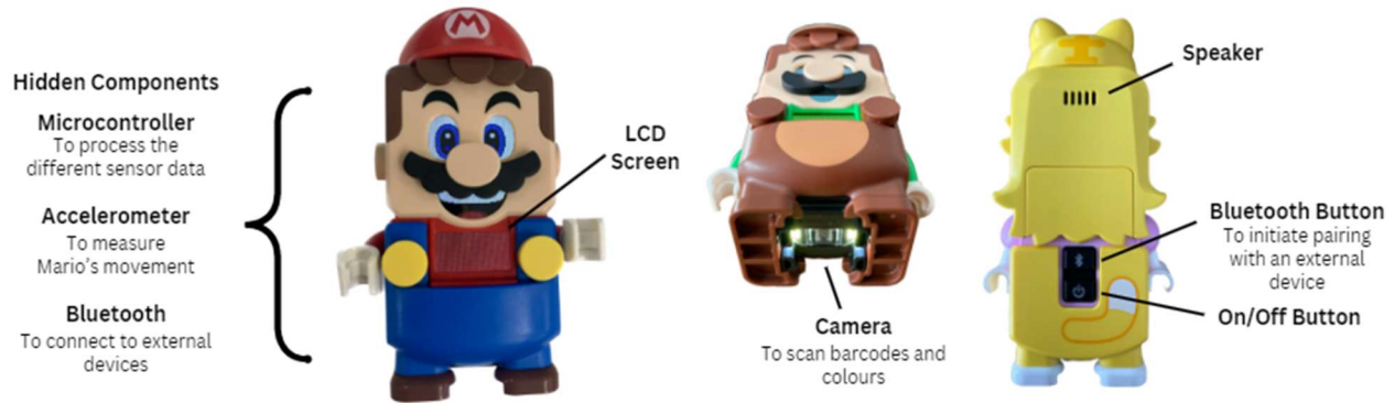
Figure 29: Diagram of the Components on the Front, Under and Back Sides of the Figurines. Left to Right: Mario, Luigi (wearing Tanooki pants) and Peach (wearing Cat pants).
