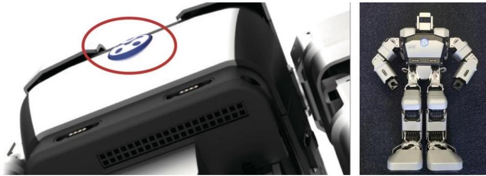
*Figure 6: On/Off button located on Buddy's chest*
