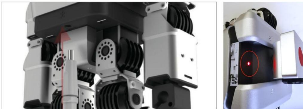
*Figure 7: Location of the battery charging indicator*
